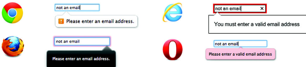
Figure 2.3 Each web browser vendor implements a different style when presenting input validation errors to the user. As more websites begin to use HTML5 form validation, users will become more familiar with the standard style of error message displayed by their browser of choice.
