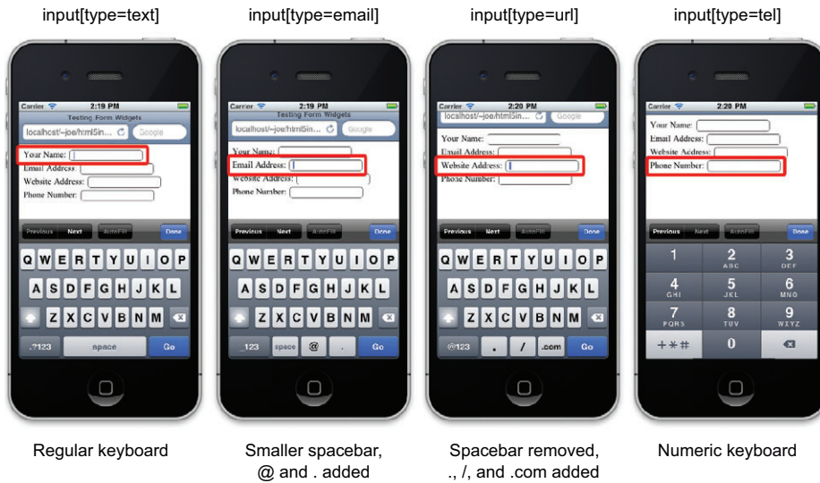
Figure 2.2 Different virtual keyboards are displayed on an iPhone for different input types—from left to right: text, email, url, and tel. Notice how symbols are added and removed for the email and url input types. An entirely different keyboard is displayed for the number input type.
