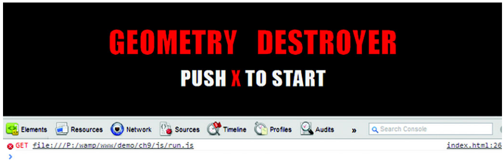
Figure 9.5 If you load up index.html and take a look at your console, it will display no errors or that run.js is missing. Know that if you've created a run.js file already, it won't fire the shown error.
