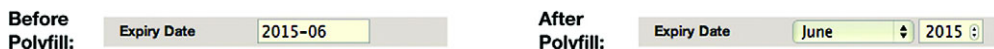
Figure 2.12 Before the polyfill has been loaded, the Expiry Date field is represented merely by a text input. After the polyfill has been loaded, the field has been replaced with a month drop-down and a year number input field. The polyfill listens for changes to these fields and populates a hidden field, which stores the month in YYYY-MM format. This hidden field will be sent to the server when the form is submitted.
