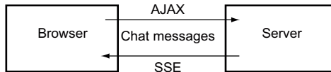
Figure 4.2 The conceptual flow of chat messages in this section's application. Messages will be sent back to the server using standard AJAX techniques, but chat messages will be received from the server through server-sent events.
