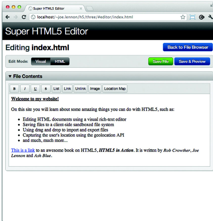
Figure 1.12 The Super HTML5 Editor application that you’ll learn to build in chapter 3 uses the designMode attribute and the Editing DOM API to allow users to edit HTML markup using a set of rich-text editing controls. The toolbar in this screenshot allows you to use Bold, Italic, Underline, Strikethrough, List, Link, and Image formatting commands on the contents of the area below the toolbar.
