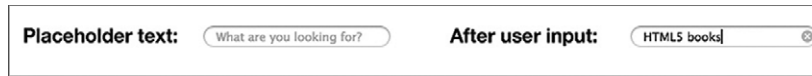
Figure 1.2 You can use the new placeholder attribute to provide a piece of text that should be displayed in a field when it's empty. This text is typically gray and will be removed when you populate the field with a value.
