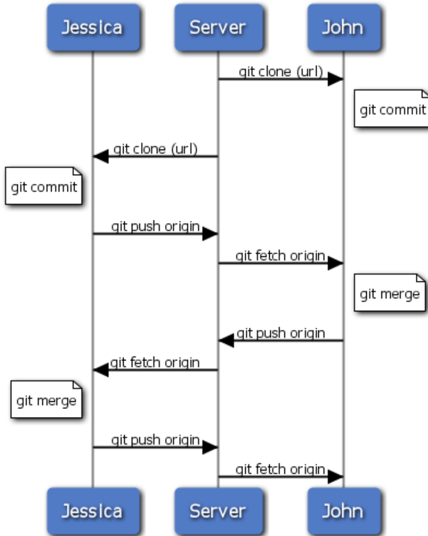
Figure 5.11: General sequence of events for a simple multiple-developer Git workflow
