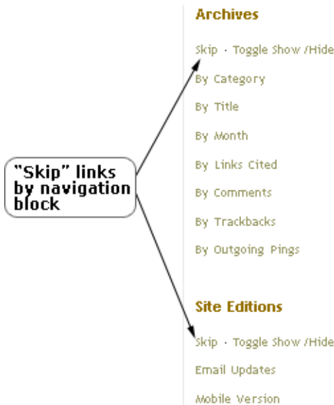
Figure 10.2. Providing skip links for each block within navigation
