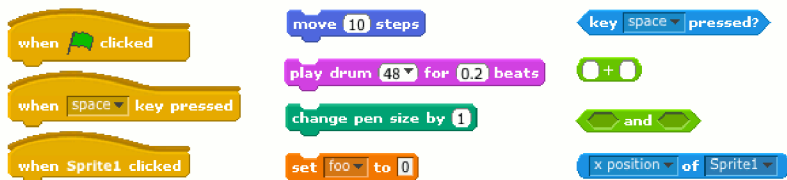
Figure 5-2. There are three types of blocks in Scratch: hat blocks (left), stackable blocks (center), and reporter blocks (right).
