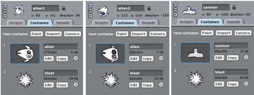
Figure 5-5. Create two costumes for each sprite, one for the normal state and one for an explosion. Name the costumes as shown here.
