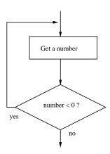
Figure 8.2: Flowchart of a post-test loop.
