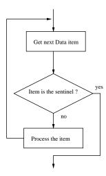
Figure 8.3: Loop-and-a-half implementation of sentinel loop pattern.
