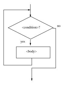
Figure 8.1: Flowchart of a while loop.
