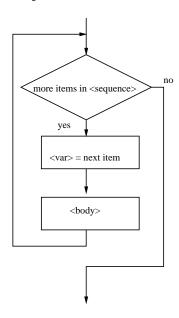
Figure 2.3: Flowchart of a for loop.
