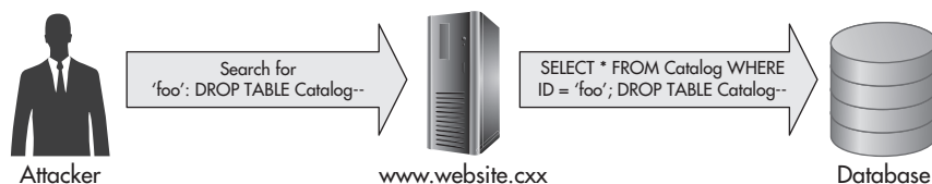
Figure 1-4 An injection attack against an application’s SQL database
