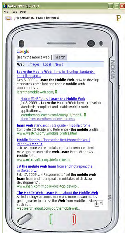
Figure 7-10. Nokia Web browser running in Nokia N97 device emulator for Series 60, 5 th Edition Platform
