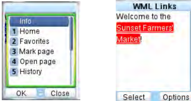
Figure 3-4. WML Browser Menu with Info Menu Item Generated from WML Do Tag in Listing 3-8
