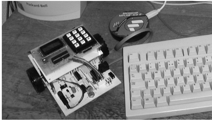
Figure 7.21: ICD 2 connected to a Derbot AGV
