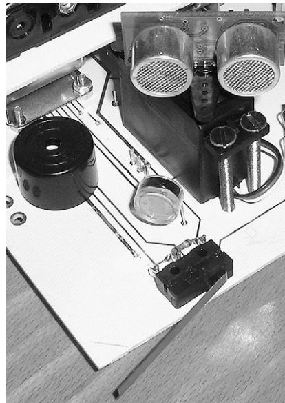
Figure 8.12: Some of the Derbot’s sensors and actuators – an ultrasonic distance sensor mounted on a Futaba servo, behind a light-dependent resistor and microswitch
