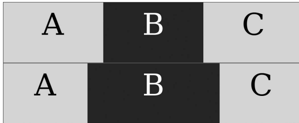
Figure 4-10: A greater flex-grow value means item B in the lower example becomes proportionally larger than its siblings.
