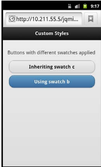
FIGURE 13.5 Buttons either inherit the swatch, or can use one that is manually set.
