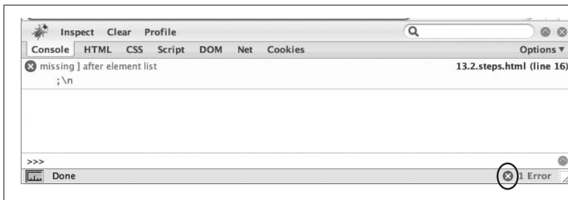
Figure 13-9: The Firebug console is the first stop for tracking down syntax and runtime errors that bring a script to its knees.
