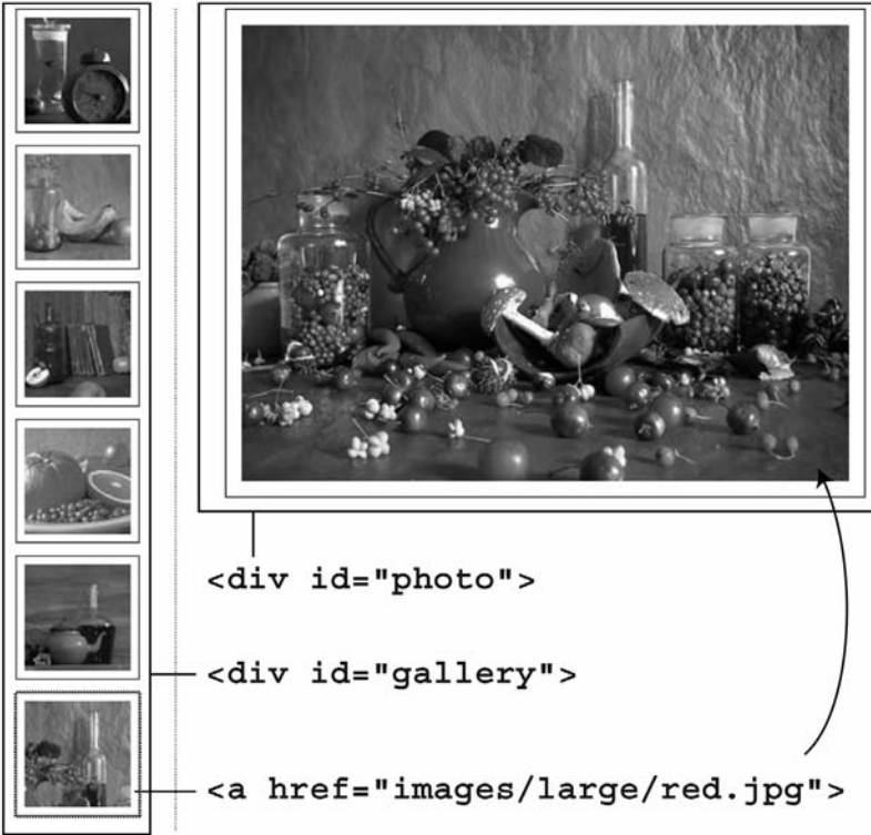
Figure 7-5: The basic structure of the photo gallery. All of the thumbnail images are wrapped in links that point to the larger version of the photo. Clicking each link will load the larger image inside a <div> tag with the ID of photo.
