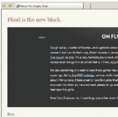
FIG 3.7: In certain Windows-based browsers, the image quickly develops too many artifacts to be readable.
