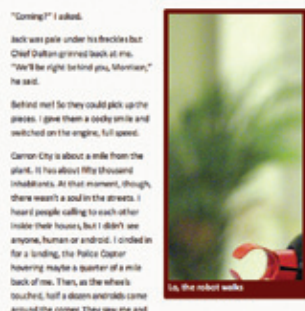
FIG 3.15: And with a dash of overflow: hidden applied to our image's container, we're left with an image that's...well, cropped. Yay, I guess?
