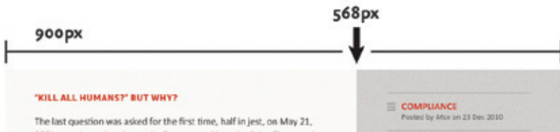
FIG 3.11: Our white column switches over to gray at the 568px mark. That’s our transition point.
