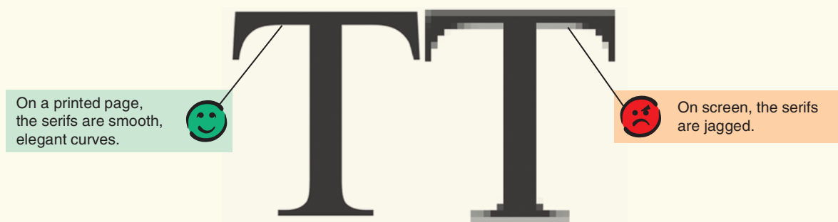
These letters are both 36-point Times New Roman, enlarged. On the left: from a book On the right: on screen.
